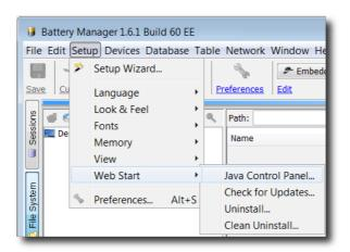
The Java Control Panel can be opened with the menu item **Java Control Panel**. The <code>javaws</code> executable must by accessible from the execution path which is normally adjusted by the Java installer automatically. Within the Java Control Panel you can list and remove currently installed applications, view JNLP files, and much more.
