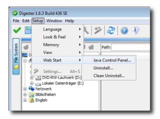
The Java Control Panel can be opened with the menu item **Java Control Panel**. The Java executable javaws must by accessible from the execution path which is normally adjusted by the Java installer automatically. Within the Java Control Panel you can list and remove currently installed applications, view JNLP files, and much more.
